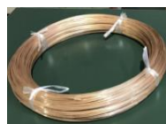
Slightly shiny surface (drawing with powder lubricant by carbide die)
