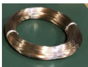
Shiny surface (drawing with liquid lubricant by diamond die)
